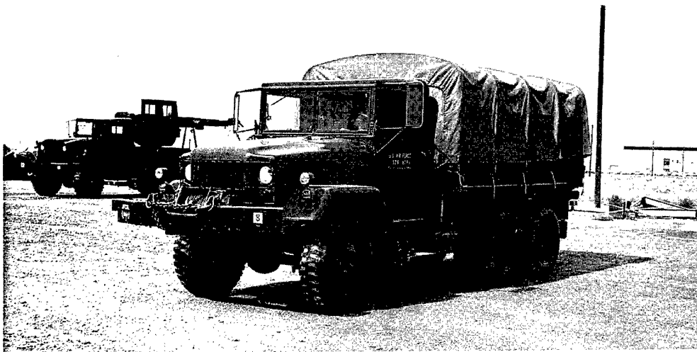
Fig. 31. An M-35 2 1/2-ton cargo truck, commonly referred to as a “six-by-six,” were used by the Holloman Balloon Branch to launch and recover anthropomorphic dummies and suspension racks at numerous locations throughout New Mexico. (U.S. Air Force photo)
